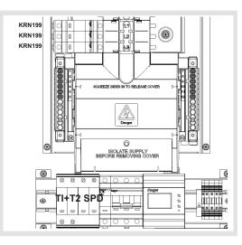
Clip the 4 module surge protection device to the dinrail next to the incomer. Fit the 3 KRN199 terminal block's to the first 3 phases on the left hand side of the busbar stack as shown above and torque to 3.5Nm.
