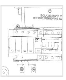
Place the copper earth component into the bottom two cage terminals of the surge protection device and secure to 3.5Nm.
