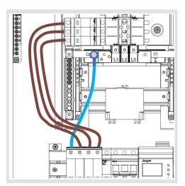
Secure the 3 brown cables to the terminals of the Surge protection device and the corresponding KRN devices L1/L2/L3 and torque to 3.5Nm.
