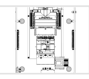
Meter installation position bottom right of the 250A TPN board, if to aperture in the bottom right hand corner please use the din rail provided to mount underneath the incomer molding and cut out where applicable and follow the phase connections below - CT fixings remain the same.
