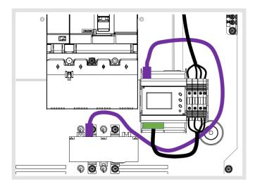
Fit the meter and fuses L3/L2/L1/N as shown above by clipping to the bracket.
