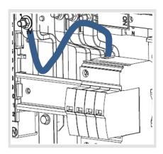
Connect Neutral cable to the neutral bar with the M5 hex Carp nut and torque to 5Nm
