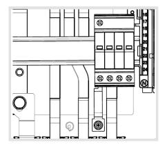
Clip surge protection device to din rail on the right hand side as shown & connect the copper earth link into the SPD and using the Hex head High Torque screw to the chassis at 5Nm 'Always install the chosen Incomer first'.
