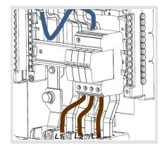
Connect the L1/L2/L3 cable lugs to the Incomer using the M8 Bolts provided making sure to use the flat washer and shake proof washer, torque to 13Nm
