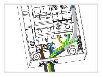
Remove the desired knockouts and fit the meter tail cable protector plates on the load and/or supply side of the enclosure.
