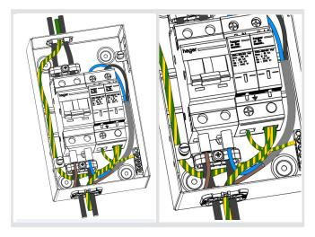
Bring the (meter tails) into the top of the enclosure including the 16mm Earth cable, terminate the L&N tails into the main switch and torque to 3.6Nm, terminate both earth cables into the Surge protection Earth connection point and torque to 3.6Nm. (Ensure Cable clamps are clamping the meter tails top and bottom)
