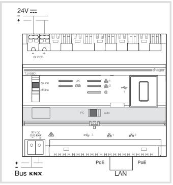
The IoT Controller can also be connected to a PoE (Power over Ethernet) network
