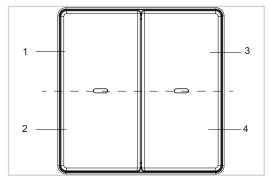
Figure 3: Button/input assignment – numbering in configuration tool 2gang
