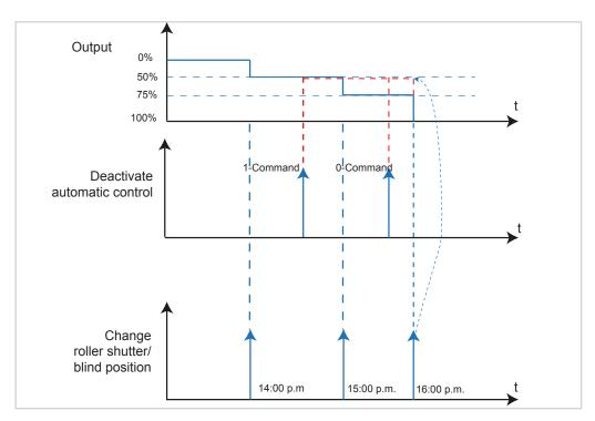
Figure 53: Signal-time diagram for Automatic control deactivation
