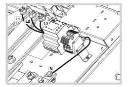
Remove the busbar shroud and fit Line & Neutral cables to the positions as shown above. Tighten to the required torque stated in the panelboard instructions.
