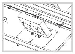
The CT Pack needs to be fitted in the cable extension box below the panelboard, plug the CT to the meter with the RJ45 cable.
