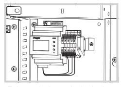
Fit the meter bracket onto the chassis using the fixings provided.
