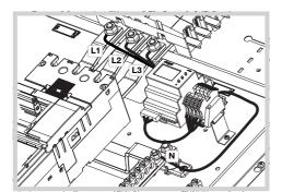
Remove the busbar shroud and fit Line & Neutral cables to the positions as shown below. Tighten to the required torque stated in the panelboard instructions.
