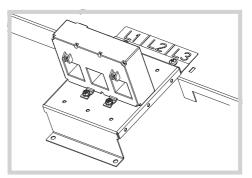
Fit the CT and bracket to the chassis and base using the fixings provide, plug the CT to the meter with the RJ45 cable.
