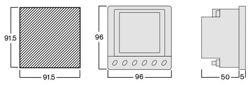
Please allow space at the rear of the meter for cable connections.
