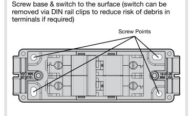
Strip/dress cables, 16/25/35mm² can be used (17mm strip length required)
