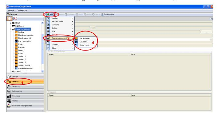
To enable domovea to provide the displays or perform energy data comparisons between periods, it is necessary to create an archive of the values measured.
