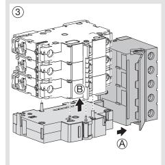
For removal of AOB from MCB, insert screwdriver, push grey lock button up.
