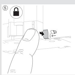
Push the grey button to comply with product standard IEC 61009-1 Annex-G. When button pushed
