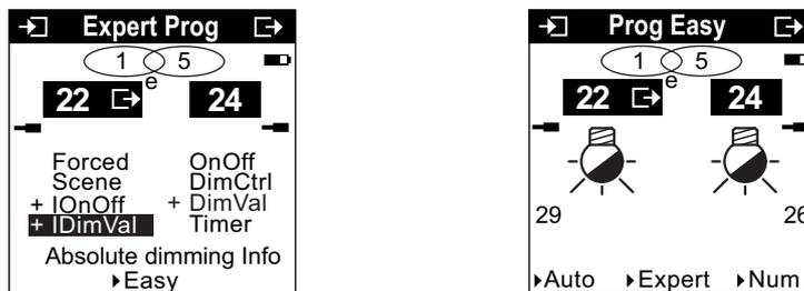
The link created this way allows operating the output of dimmer TXA 215 as a slave of TXA 210 and displaying the common lighting level value of the 2 outputs on the LCD display of the TXA 215.
