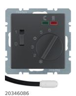
Thermostat, NO contact, Cen. plate, f. heat., rocker switch, ext. temp. sen., Q1/3, ant.
